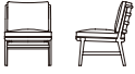
The sensual ladder back lounge I-743 lounge chair W573 × D690 × H778 × SH438
